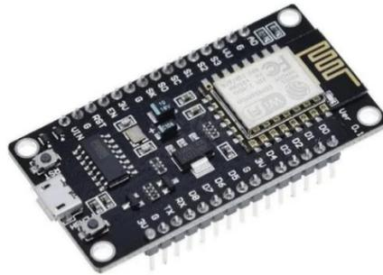
Figura 5. NodeMCU
